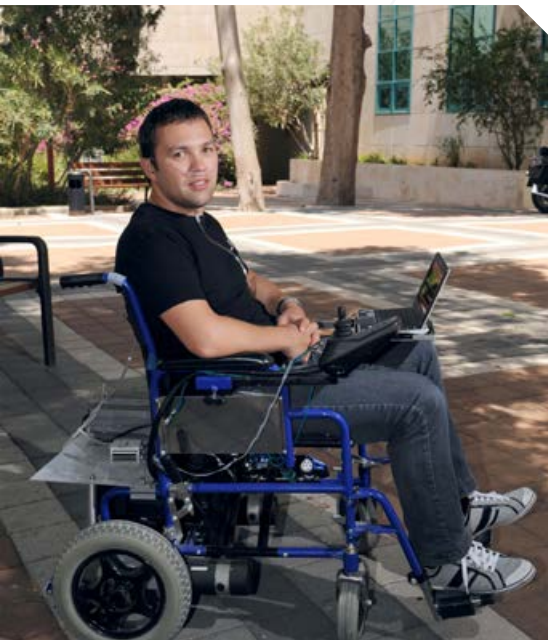
Dr. Anton Plotkin in the lab of Prof. Noam Sobel, testing the sniff-controlled motorized wheelchair.
