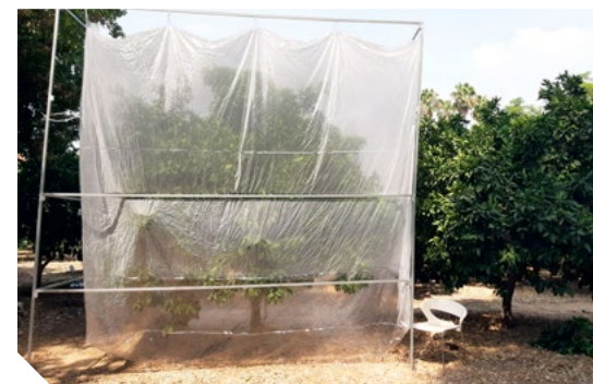
The Klein lab isolated this lemon tree from its neighbors to measure its carbon and water budgets.
